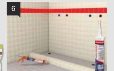
6. Finally, seal the intersections with **DOMOSIL-MICRO**.
